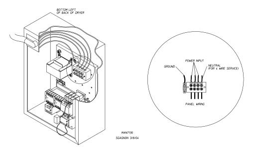
The neutral will only be used on 4-wire service. This is typical for 380-416V, 50 Hz.
